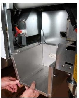
Figure 2: Position the melter.
