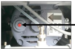
Filter Pump Reset Switch
