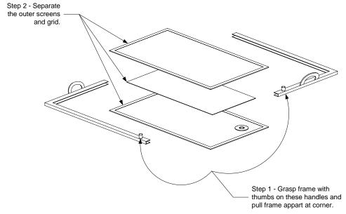
2. Separate the outer screens and grid.
