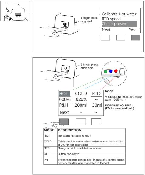
Volumes must be calibrated and machine must be notified of Chillers presence, go to page 14
