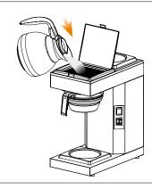
Lift up the tank lid and pour in a decanter of fresh tap water.
