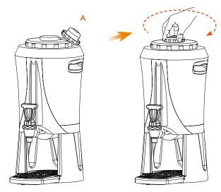
To keep temperature and aroma, put the lid (A) back on the serving station immediately after the brewing.
