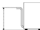
**IN THIS CASE, THE DRAIN CONNECTION MAY BE NO HIGHER THAN 1 M. ALWAYS CHECK THAT THE DRAIN WORKS PROPERLY AND IS NOT BLOCKED.**
